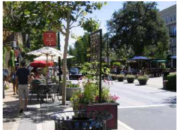
No on-street parking, expansive sidewalks and flush surface (San Jose, California)
