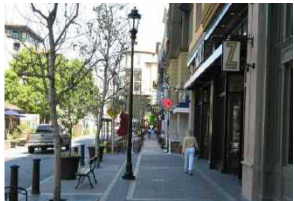
Sidewalk organized according to best practice functional zones: building edge, pedestrian thru zone, furniture zone and curb / parking zone (San Jose, California)
