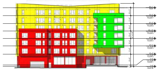
BUILDING MATERIAL IDENTIFICATION ELEVATION - SOUTH OVERALL 2
