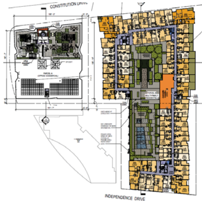
Figure 6. The proposed extent of landscape vegetation to be planted on green roofs on the project site.
