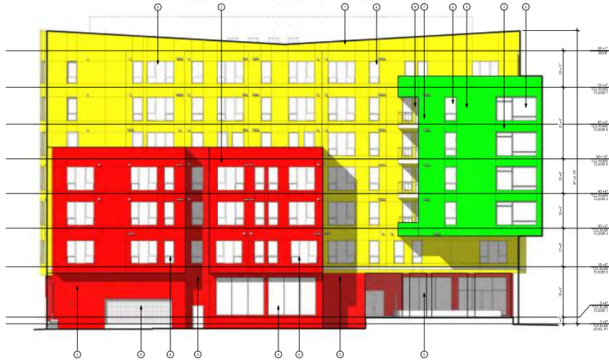
BUILDING MATERIAL IDENTIFICATION ELEVATION - SOUTH 1 1/8" = 1'-0"
