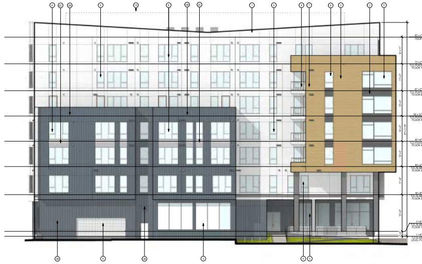
BUILDING MATERIAL COLOR ELEVATION - SOUTH 1 10' = 1" = 0'
