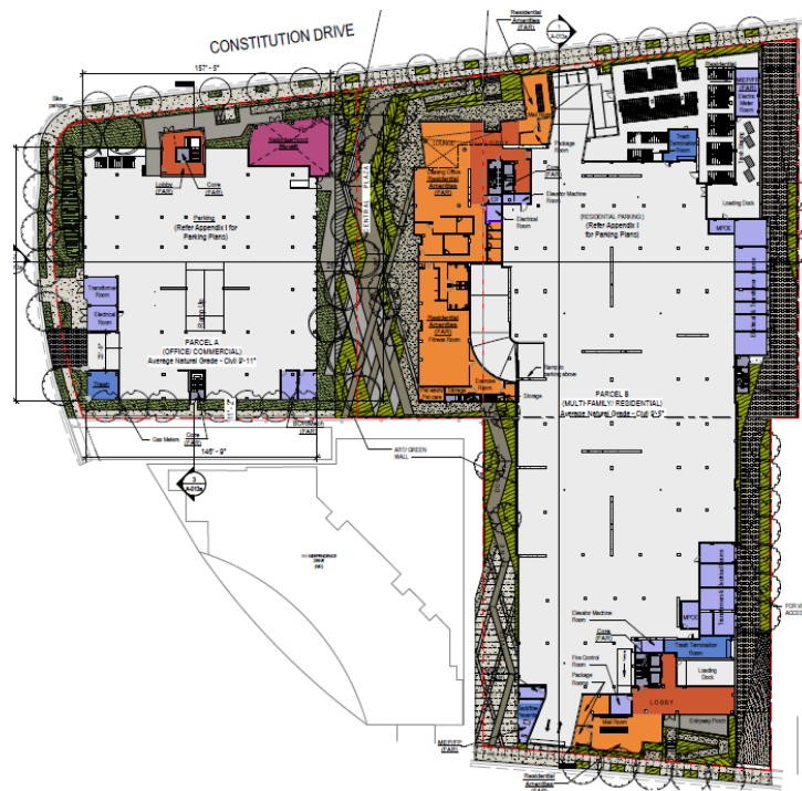
Figure 5. The proposed extent of landscape vegetation on Level 1 of the project site.
