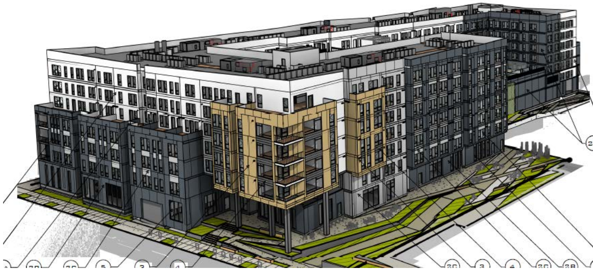
Figure 2. The proposed apartment building (MF-1) incorporates opaque wall panels, overhangs, shadow boxes, and window mullions. These features help the building appear as a solid structure to birds, and reduce the likelihood of collisions.
