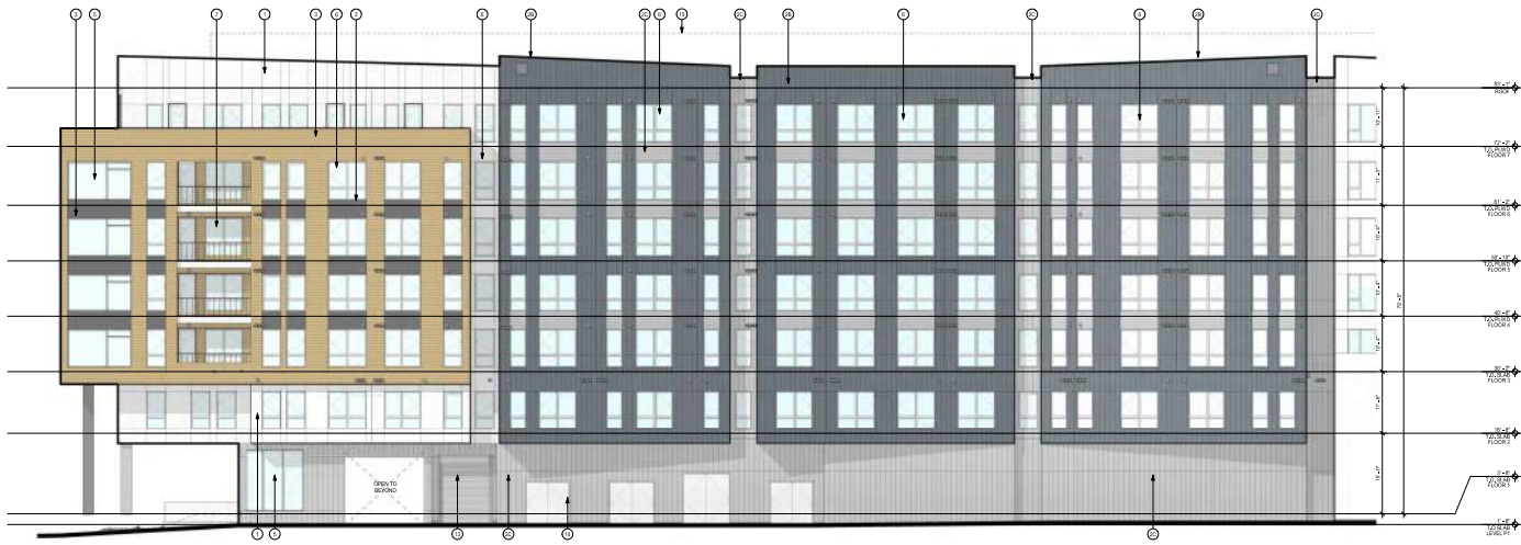
BUILDING MATERIAL COLOR ELEVATION - EAST A 2 1/8" = 1'-0"
