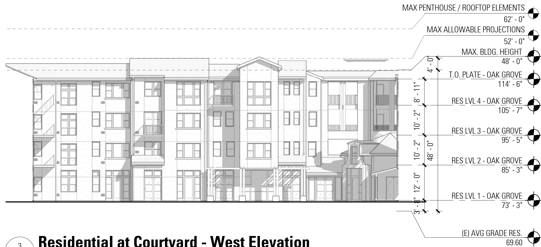
3 Residential at Courtyard - West Elevation A4.07 1/16" = 1'-0"
