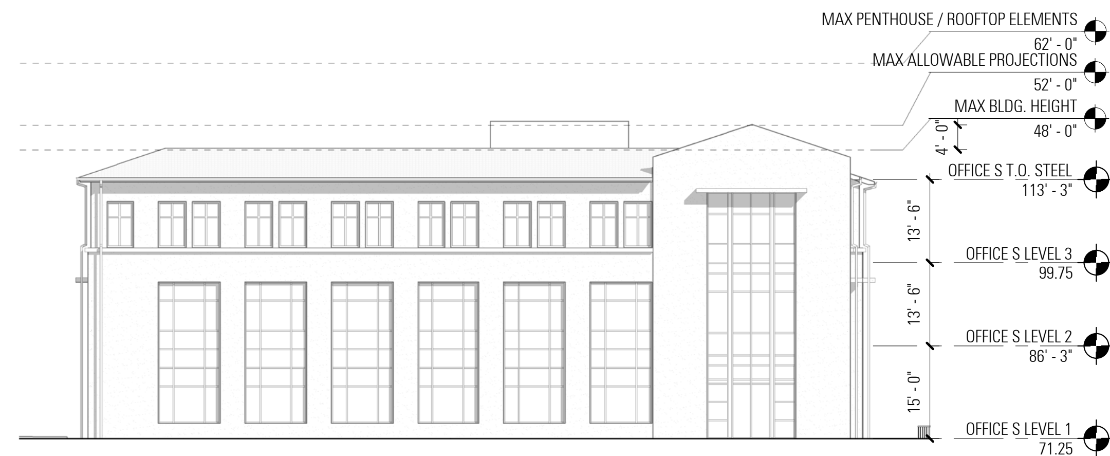
2 A4.03 South Office - Rear East Elevation 1/16" = 1'-0"
