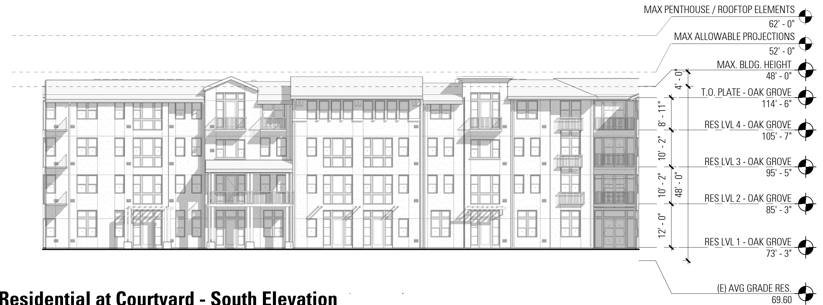
2 Residential at Courtyard - South Elevation A4.07 1/16" = 1'-0"
