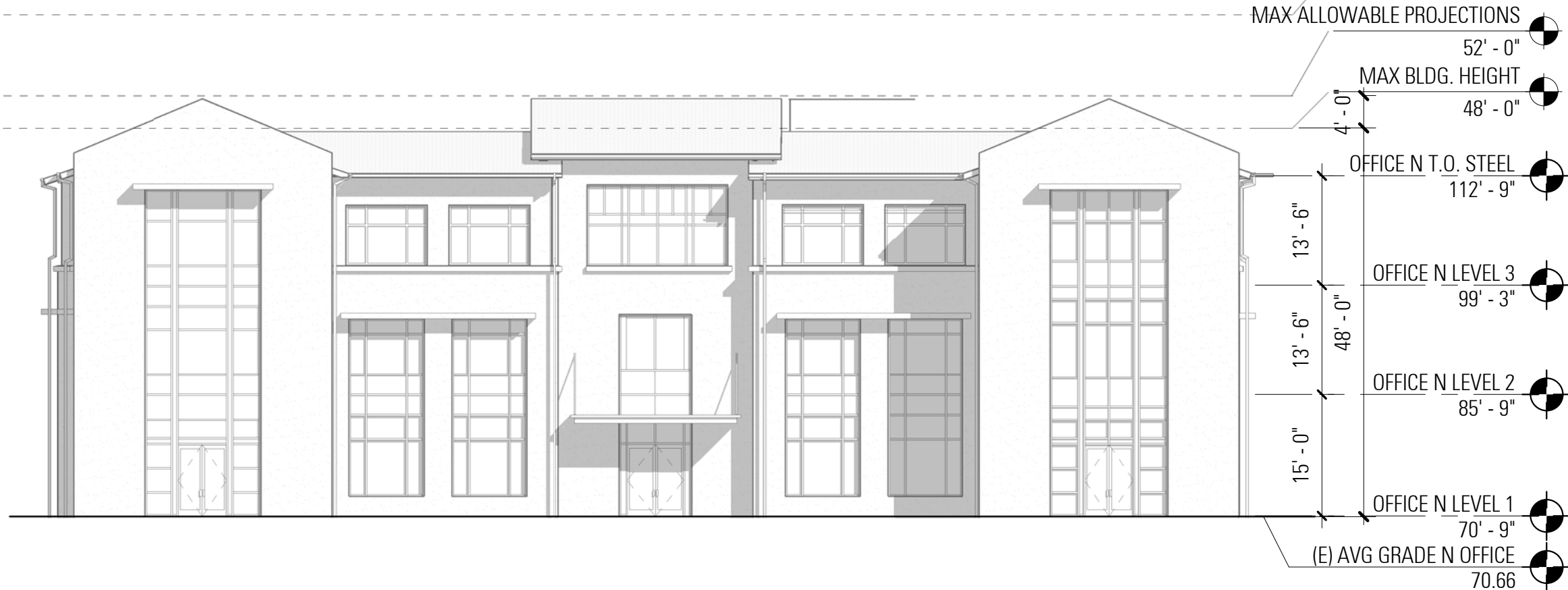
2 North Office - Rear East Elevation A4.02 1/16" = 1'-0"
