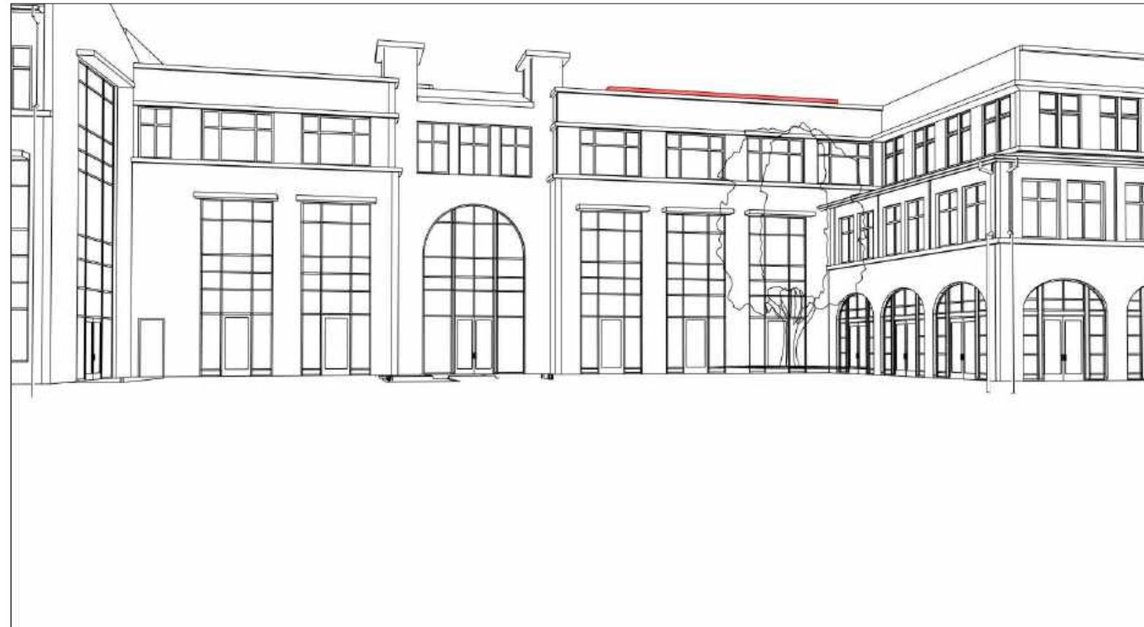
4. Perspective (oblique) view from North Office Building Plaza Entry looking toward South Office Building Entry. Cement Plaster Screen (in red) to conceal rooftop mechanical air handling unit.
