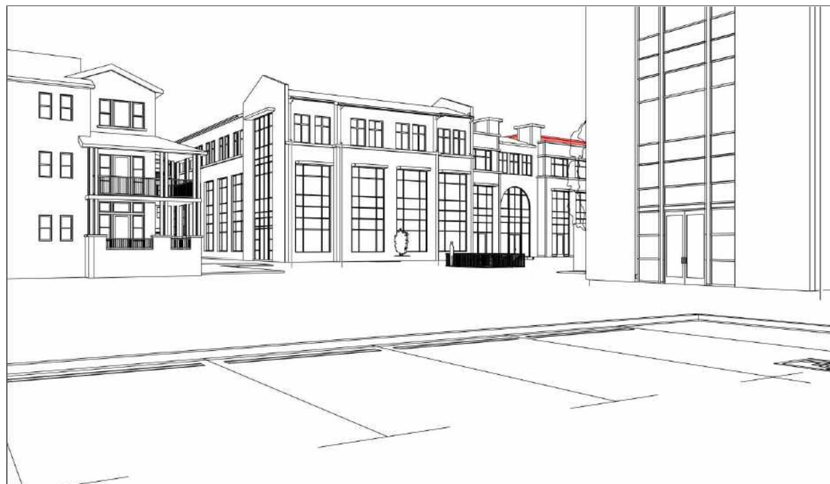
3. Perspective (oblique) view from North Office Building surface parking lot looking toward South Office Building Entry. Cement Plaster Screen (in red) to conceal rooftop mechanical air handling unit.
