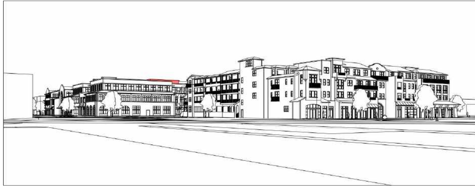
5. Perspective (oblique) view from El Camino Real, south of Oak Grove Ave. Cement Plaster Screen (in red) to conceal rooftop mechanical air handling unit.
