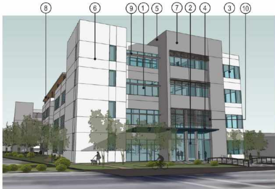
② GLASS (LOBBY), LOW-E, CLEAR DOUBLE GLASS (BIRD SAFE GLASS)
