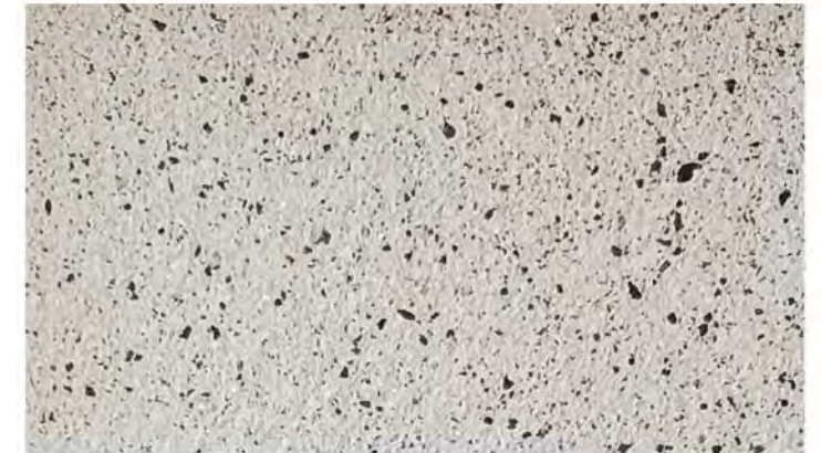
⑥ GFRC, SANDBLASTED, SMOOTH: COLOR TO MATCH DUNN EDWARDS RECLAIMED WOOD
