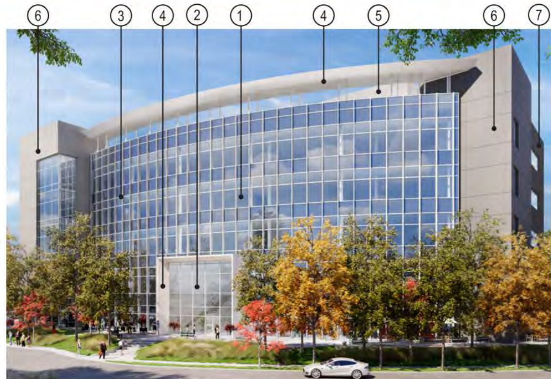
② GLASS (LOBBY), LOW-E, CLEAR DOUBLE GLASS (NON-BIRD SAFE GLASS)
