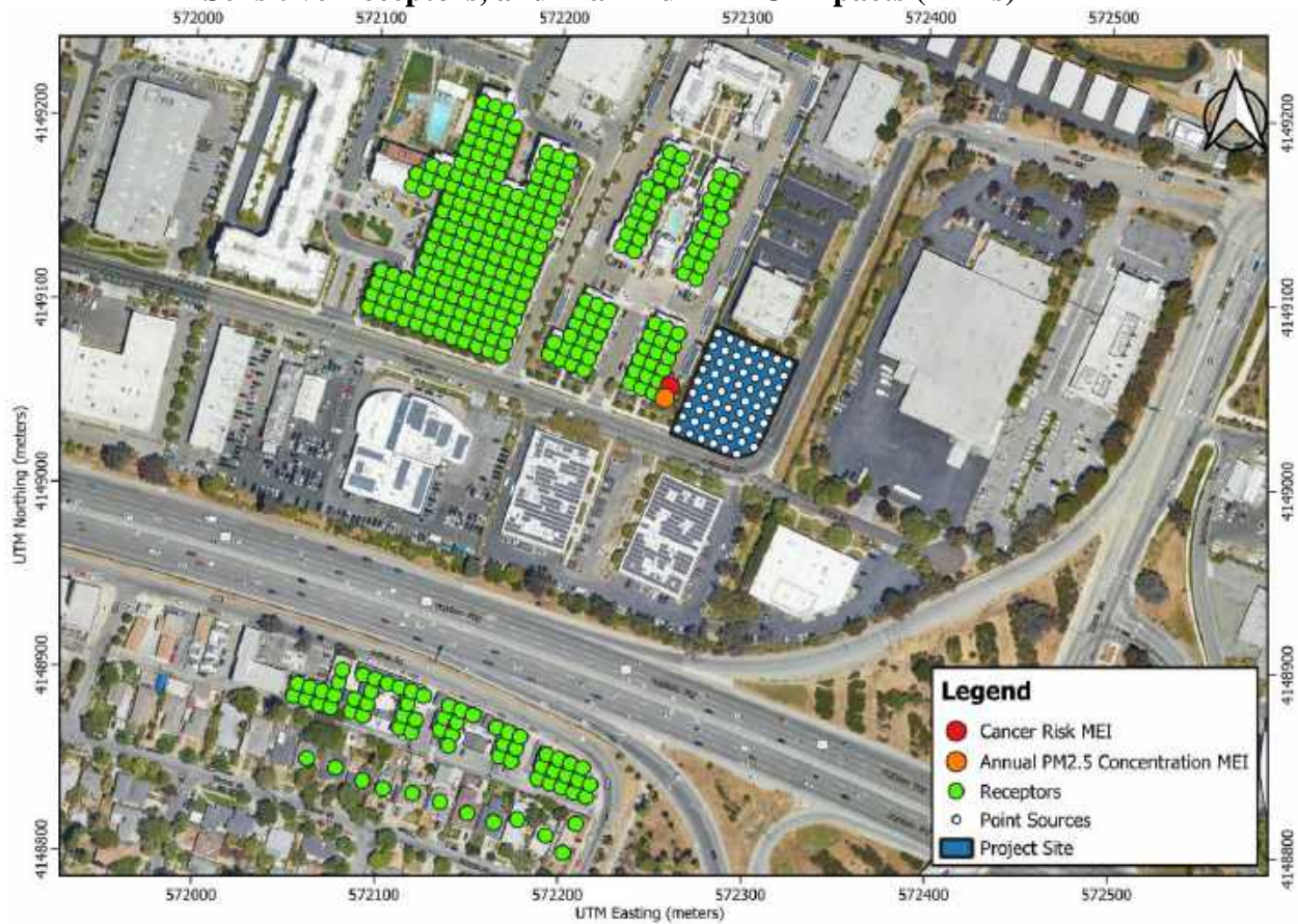
Figure 1. Locations of Project Construction Site, DPM Point Sources, Off-Site Sensitive Receptors, and Maximum TAC Impacts (MEIs)
