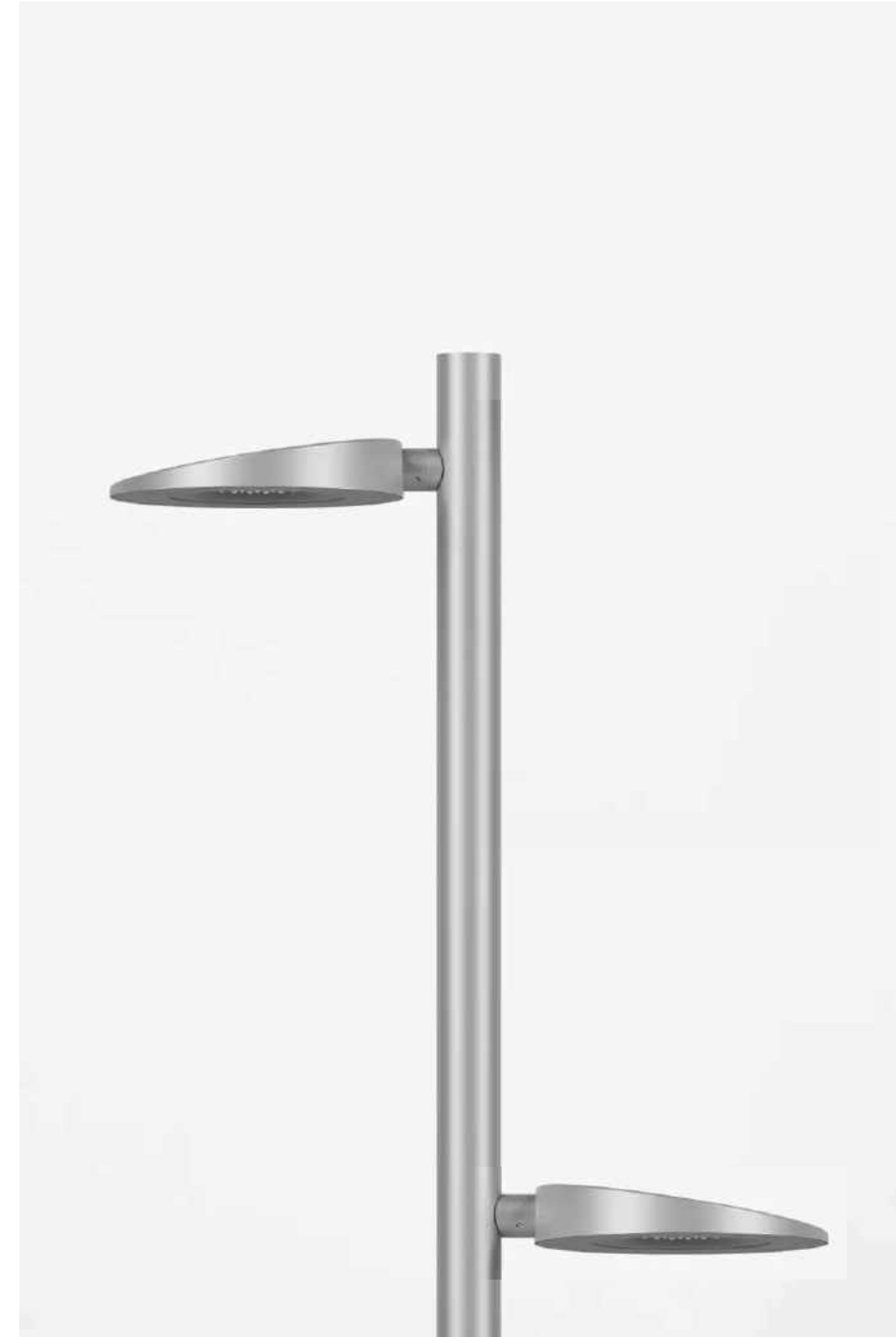
MANUFACTURER: LANDSCAPE FORMS MODEL SERIES: SLOPE AREA LIGHT POLE HEIGHT: 25'-0" TYPICAL O.C. SPACING: 85'-0" CONDITION: ROADWAY ADJACENT TO PEDESTRIAN PATH
