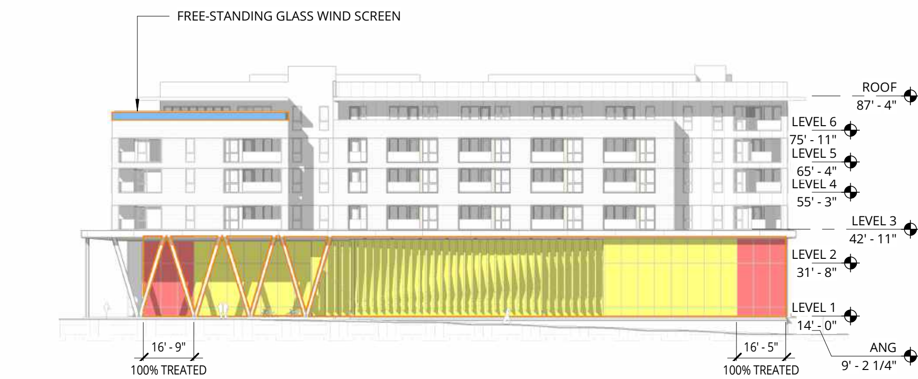
1 NORTH ELEVATION - MAIN ST. 1/32" = 1'-0"
