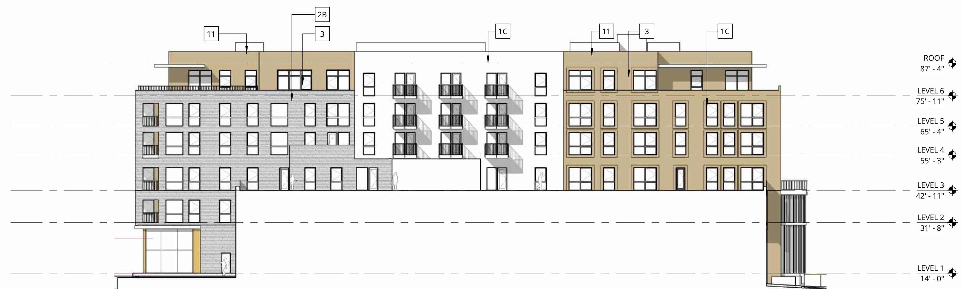
2 CENTRAL COURTYARD - SOUTH ELEVATION 1" = 20'-0"
