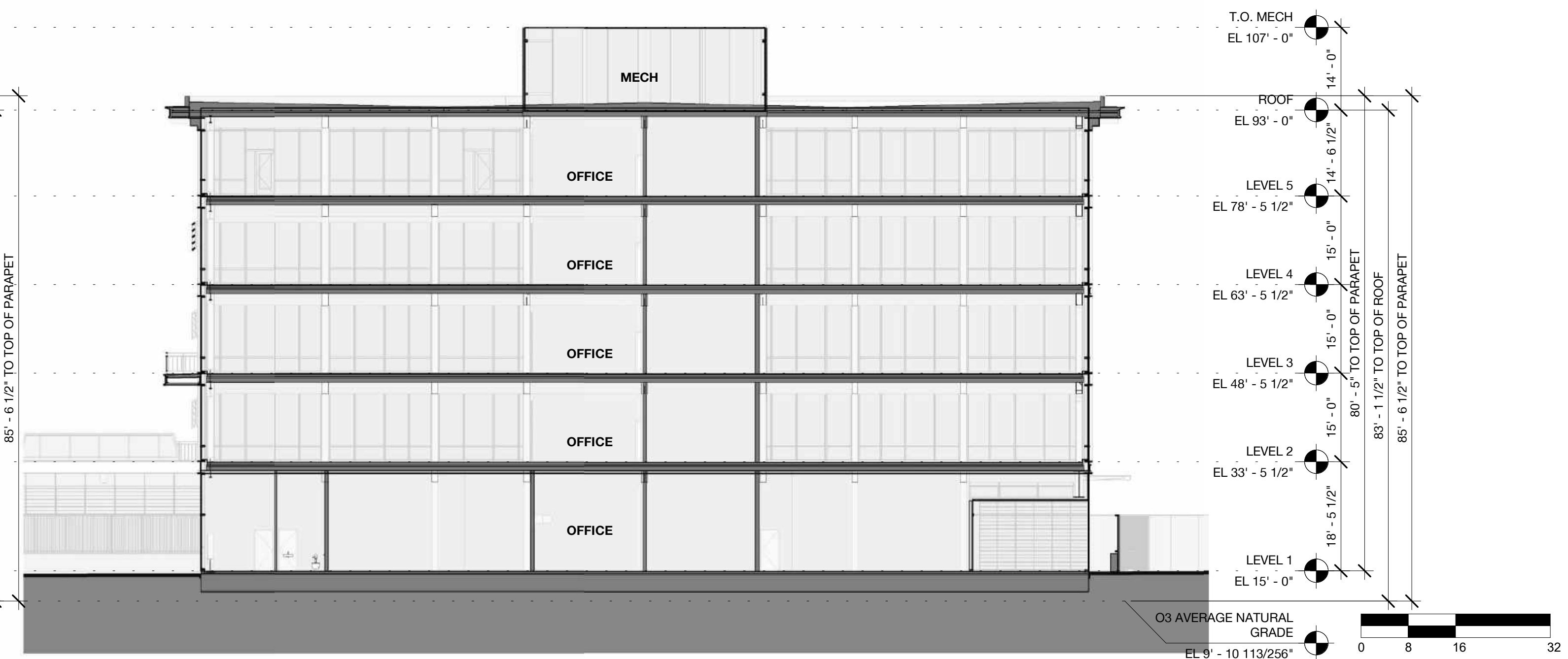
5 Building 03 - Transverse Section 1 - 1/16 1/16" = 1'-0"
