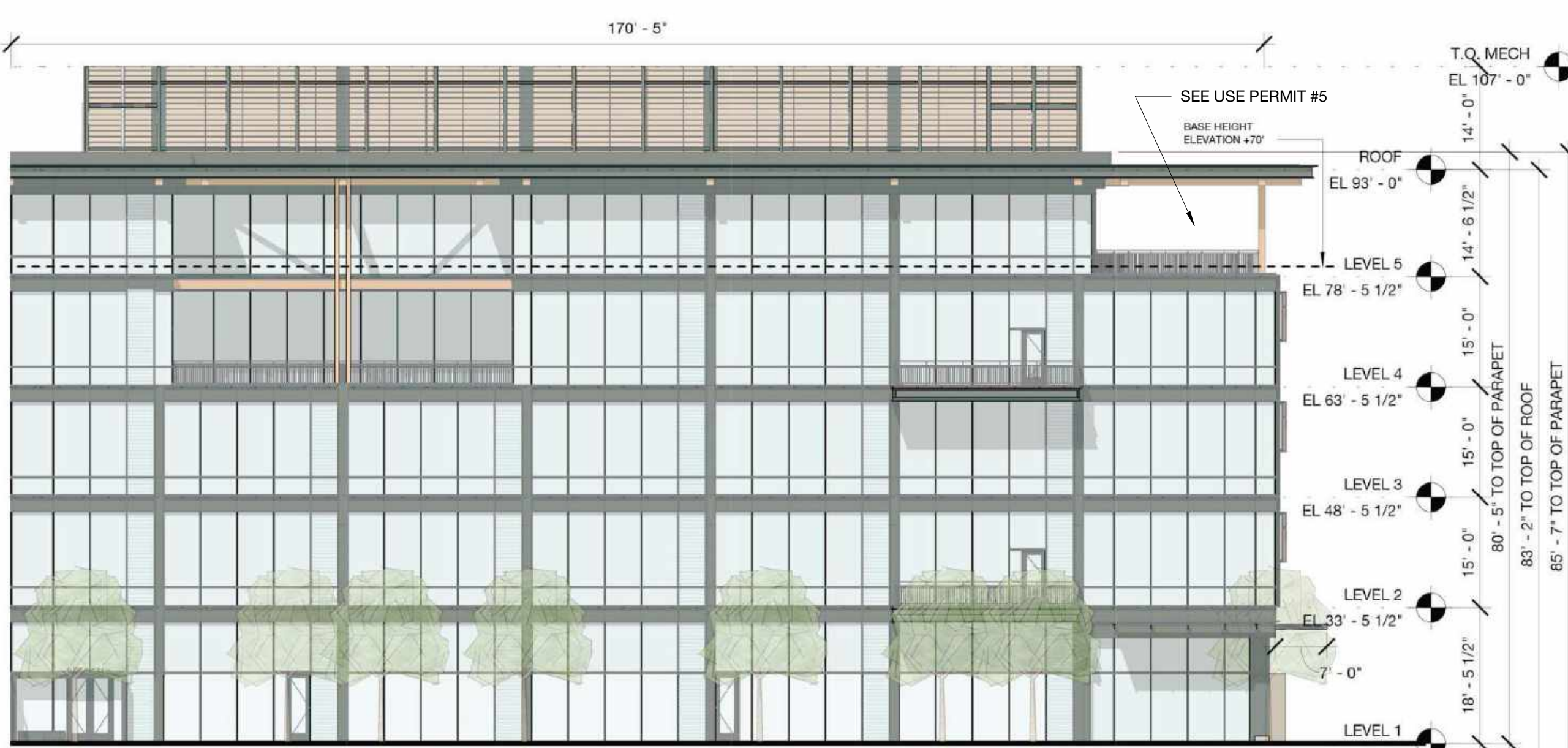
3 Building 05 - North Elevation A- 1/16" = 1'-0"
