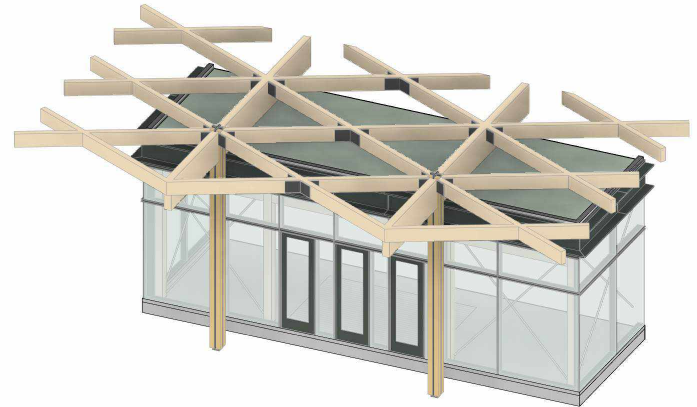
4 Entry Pavilion Enclosure - Axon 3/8" = 1'-0"
