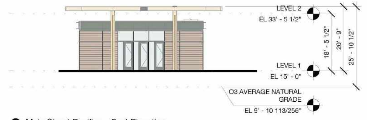
2 Main Street Pavilion - East Elevation 1/16" = 1'-0"
