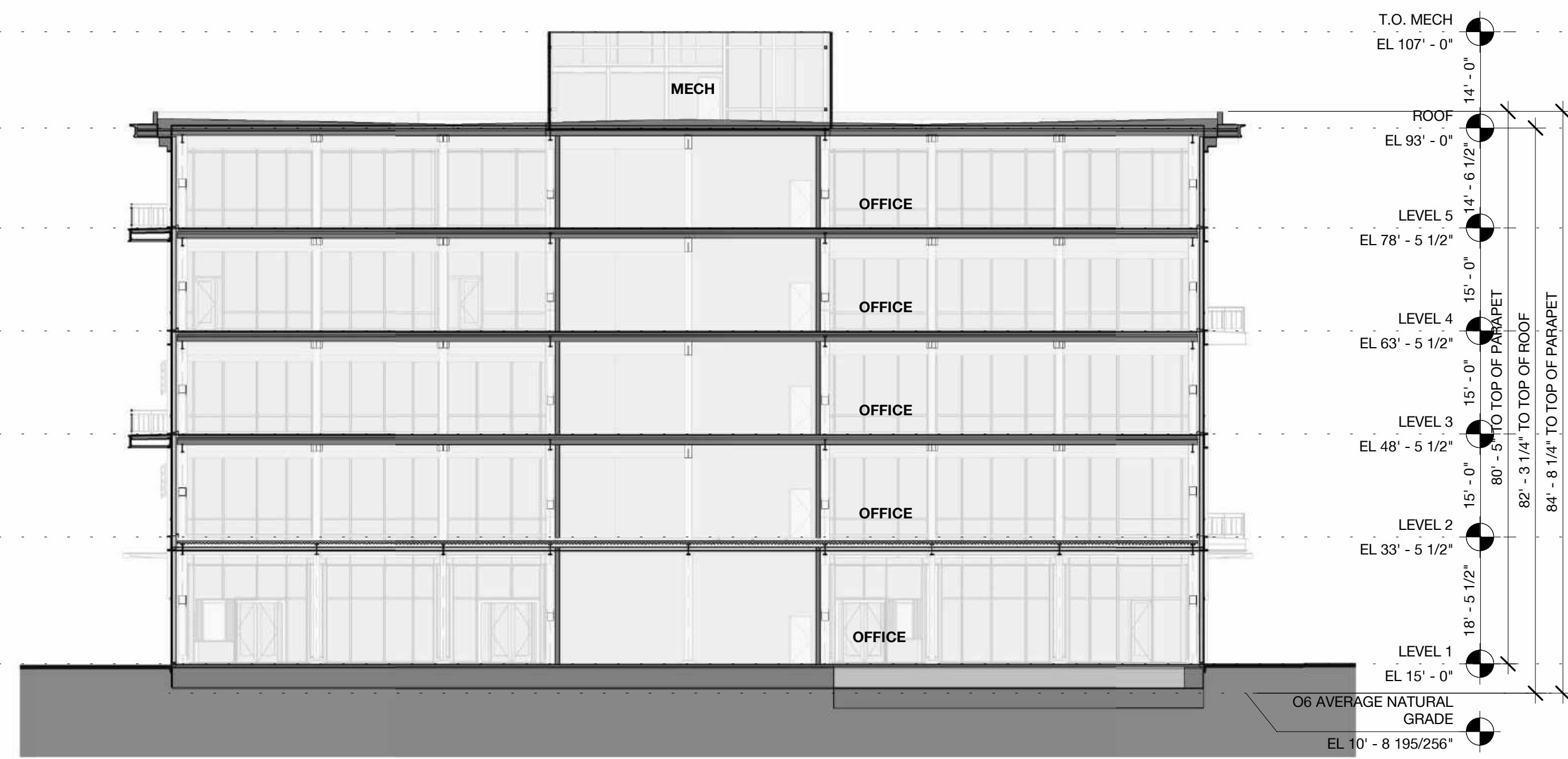
6 Building 06 - Transverse Section 2 - 1/16 1/16" = 1'-0"
