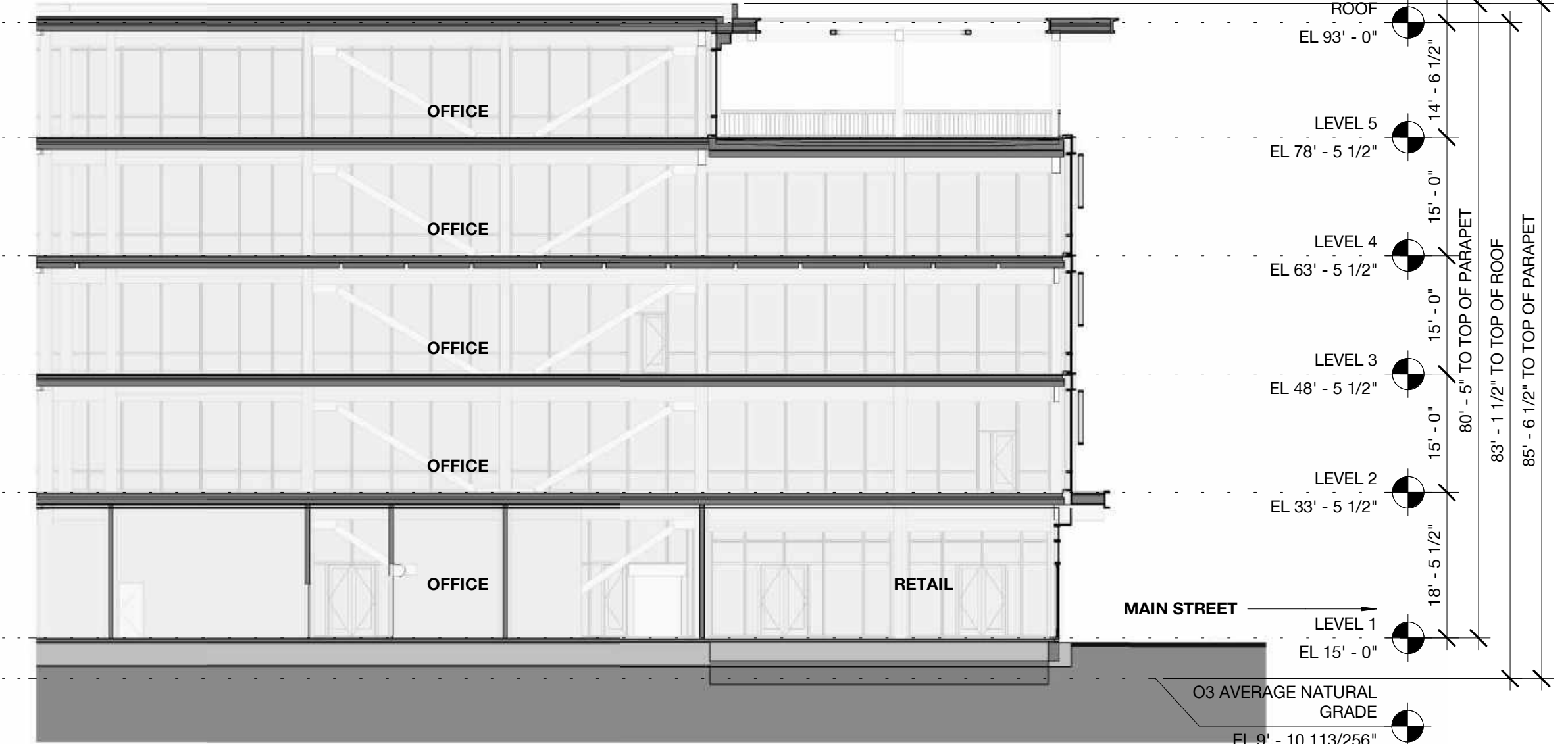
3 Building 03 - Longitudinal Section 2A - 1/16 1/16" = 1'-0"
