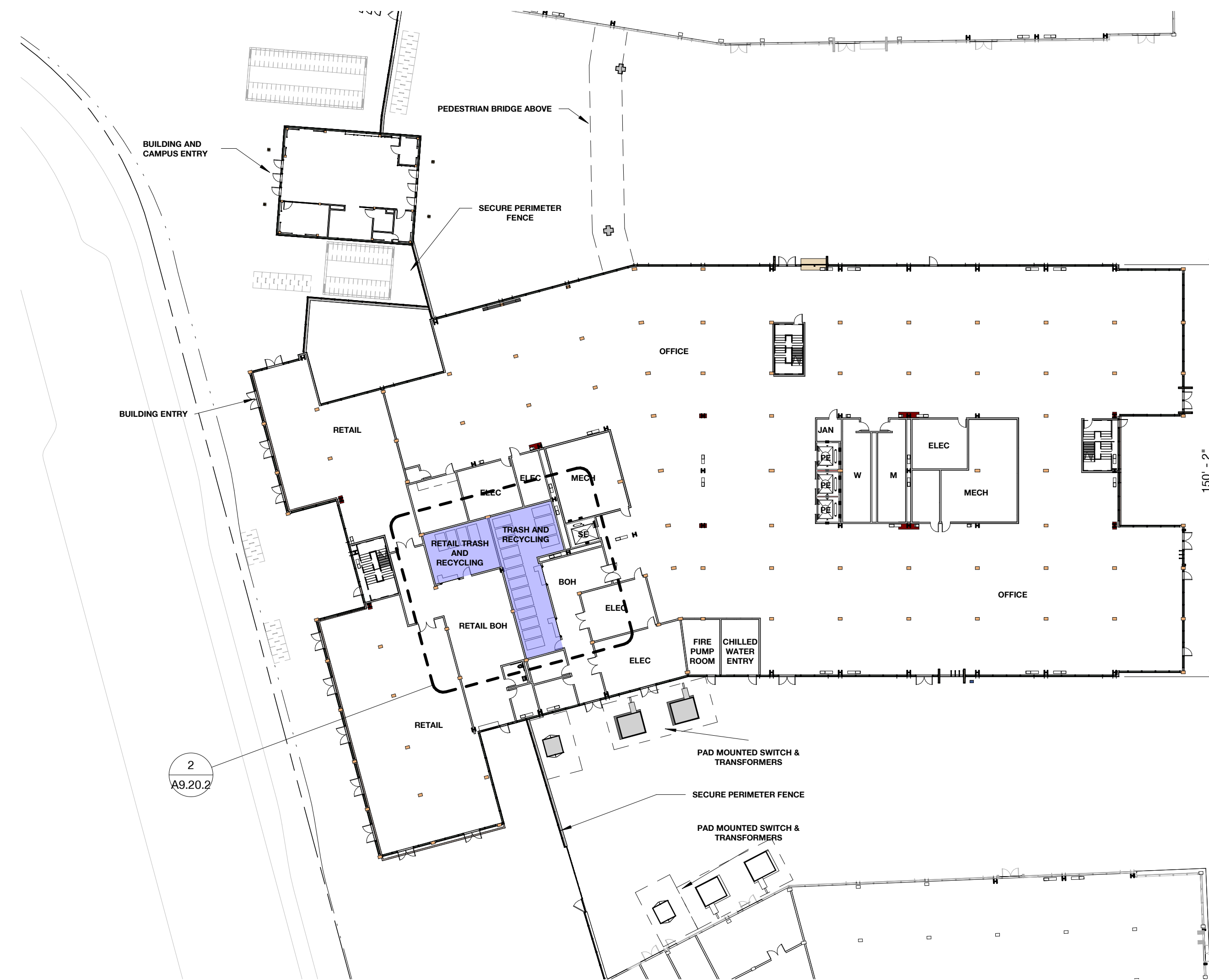
1 Building 03 - Level 1 Trash Removal 1/32" = 1'-0"
