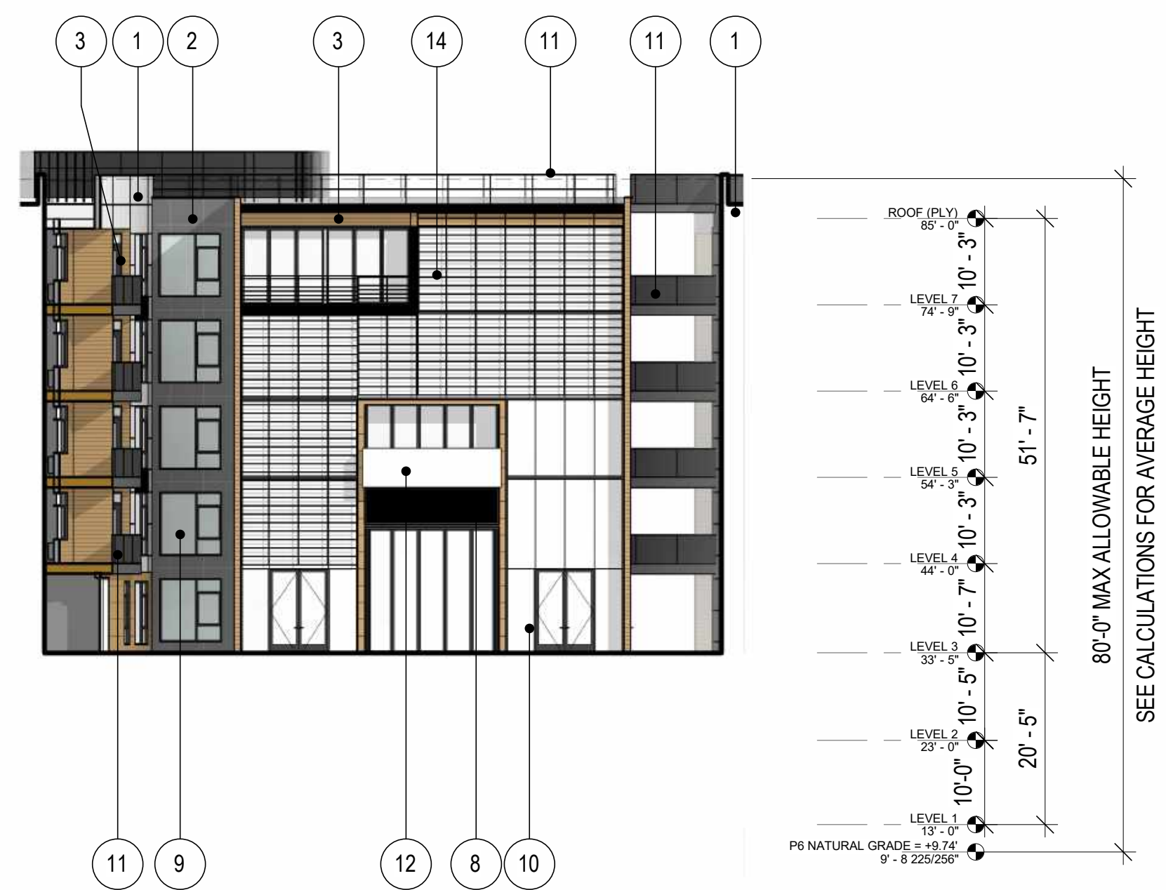
P6 - WEST COURTYARD ELEVATION #2 1/16" = 1'-0" ②
