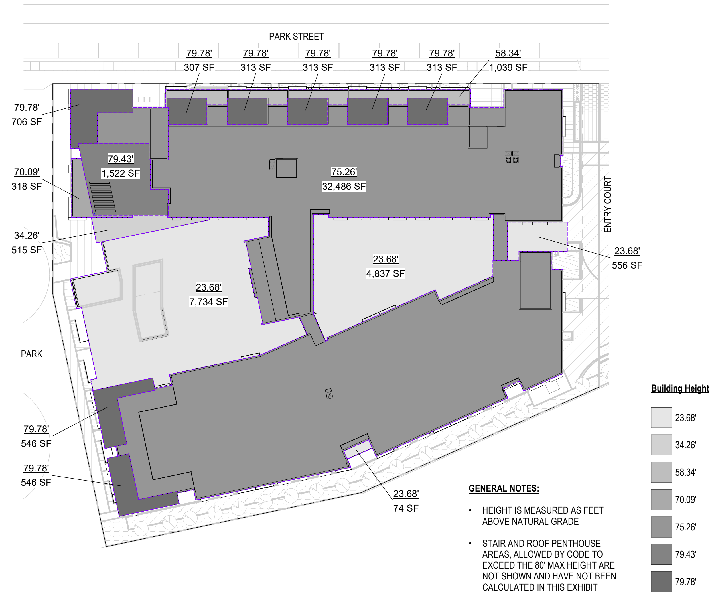
P6 - BUILDING HEIGHT CALCULATION - ROOF 1 1" = 30'-0"
