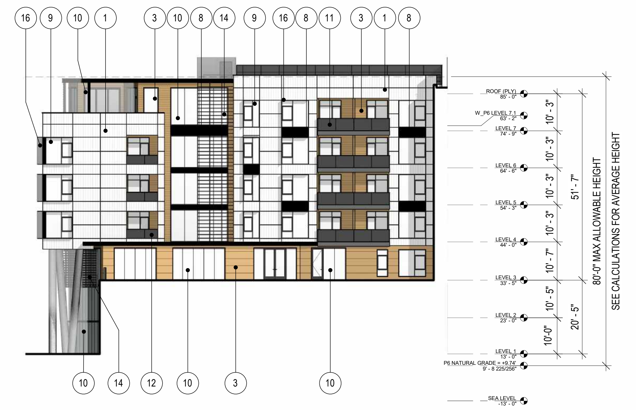
P6 - WEST COURTYARD ELEVATION #1 1/16" = 1'-0" ①
