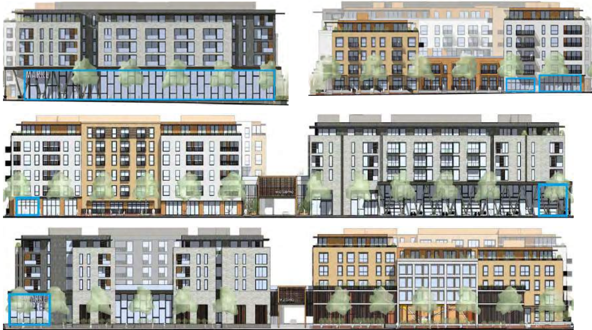
Figure 9. An example mark-up of areas (shown in blue) that would be required to be treated on north (top left), south (top right), east (middle) and west (bottom) facades of the conceptual Parcel 2 residential/mixed-use building to ensure that avian collisions are less-than-significant. Transparent glass corner delineations are estimated; these corners should be treated as far from the corner as it is possible to see through the corner. Free-standing glass railings are not indicated on this figure but are required to be treated in all locations.
