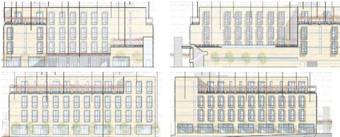
Figure 5. The conceptual east (top left), north (top right), west (bottom left), and south (bottom right) facades of the hotel.
