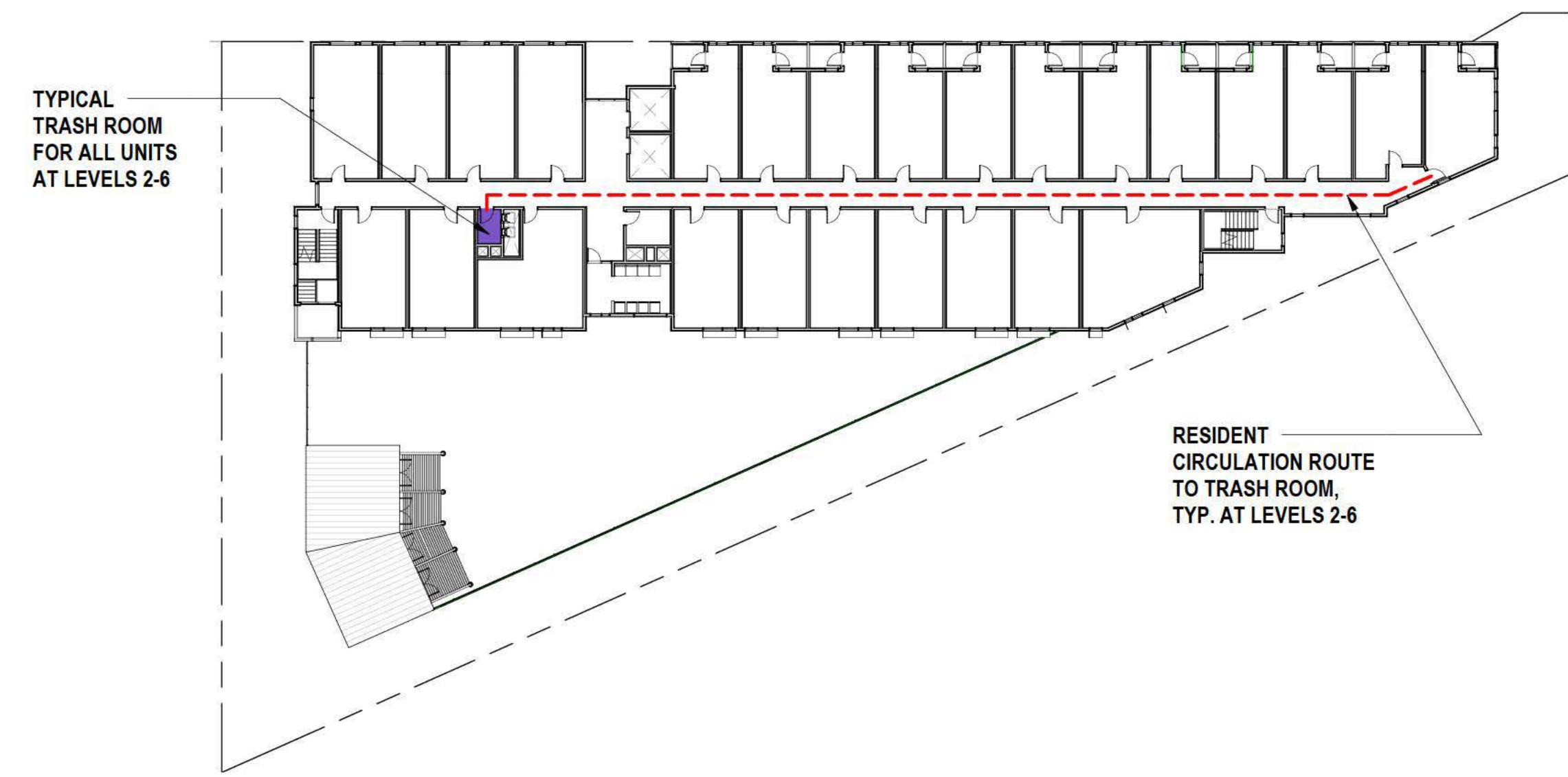
LEVEL 2-6, TYP. - REFUSE, RECYCLING & ZERO WASTE DIAGRAM 1" = 30'-0" ②
