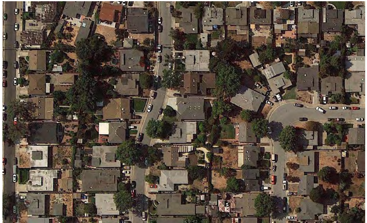
▲ This aerial photo illustrate the impervious area that generates runoff from low-density residential sites.
