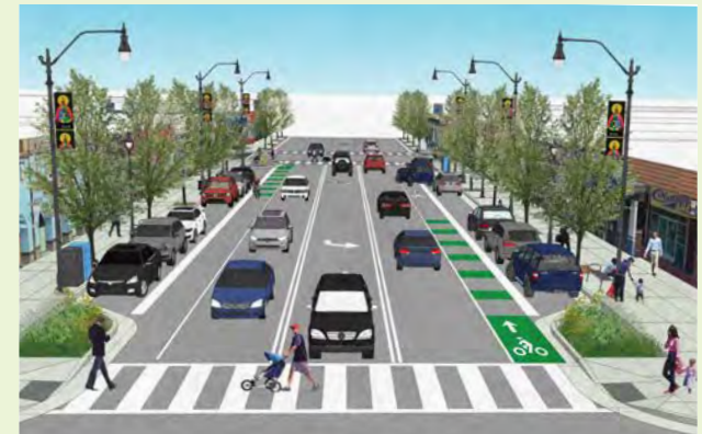
▲ Preliminary redesign of a typical block of Middlefield Road as a sustainable street with green and complete streets elements. This design reduces vehicle lanes and changes the parking configuration to widen sidewalks; add street trees, furnishings, and corner stormwater curb extensions; and designates bike lanes.
