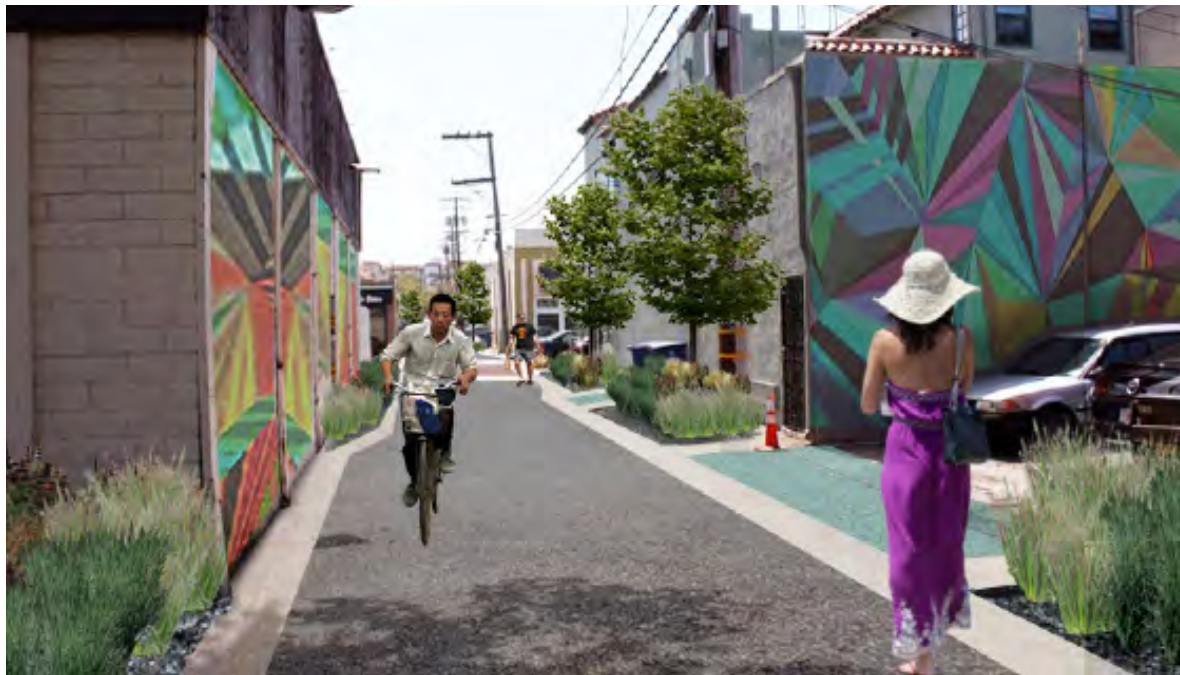
▲ RETROFIT OPPORTUNITY: The same commercial/mixed use alley retrofitted with stormwater planters and pervious paving. Colored bands of pavement can define the vehicle travel way from parking and utility areas, and emphasize pedestrian walkways and spaces. The alley's alignment offset can aid in calming traffic.
