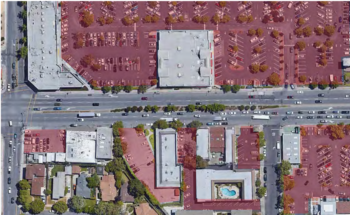
▲ The red areas superimposed on this aerial photo illustrate the impervious area that generates runoff from large and small-scale parking lots.
