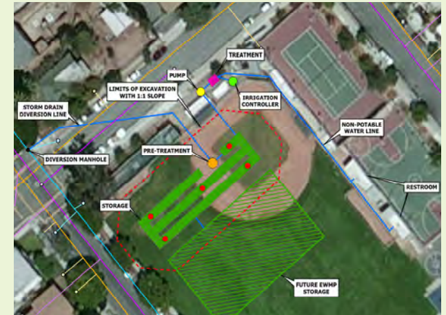
▲ Stormwater runoff and dry-weather discharge from a 50-acre urbanized watershed is diverted from flowing into Santa Monica Bay and instead treated, stored, and reused for irrigation and toilet flushing.
