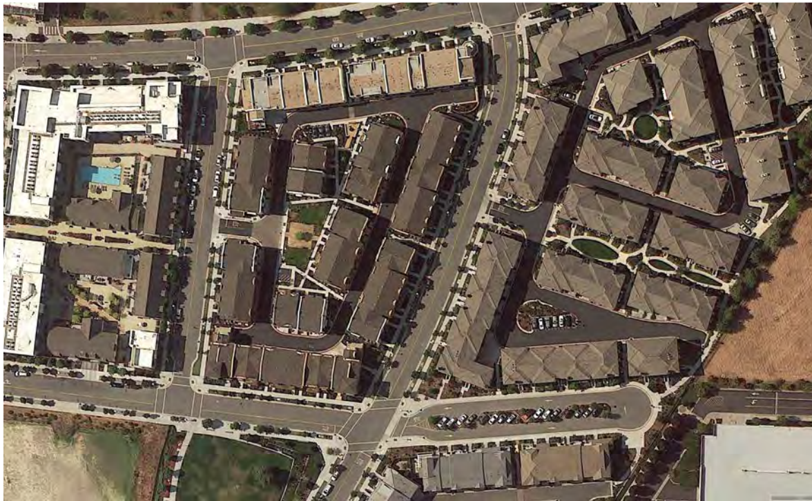
▲ This aerial photo illustrates the impervious area that generates runoff from high-density residential/mixed-use sites.
