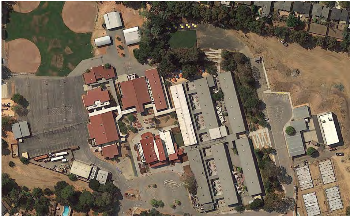
▲ This aerial photo illustrates the impervious area that generates runoff from a typical school campus.
