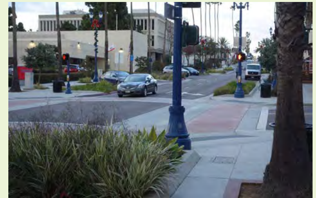
▲ Curb extensions provide green buffer zones at this intersection and also break up parking pavement along the street.
