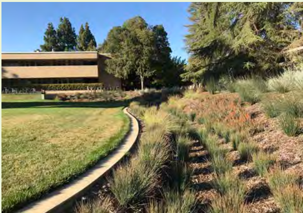
▲ EXAMPLE: An example park space rain garden captures site and sidewalk runoff and features low-water plant communities.
