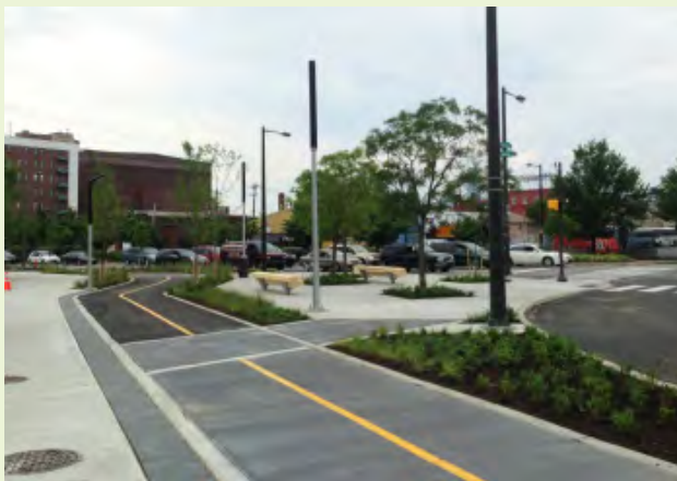
▲ EXAMPLE: Pavement materials and colors distinguish raised two-way cycle track and adjacent sidewalk. Landscape buffer from plaza and street.
