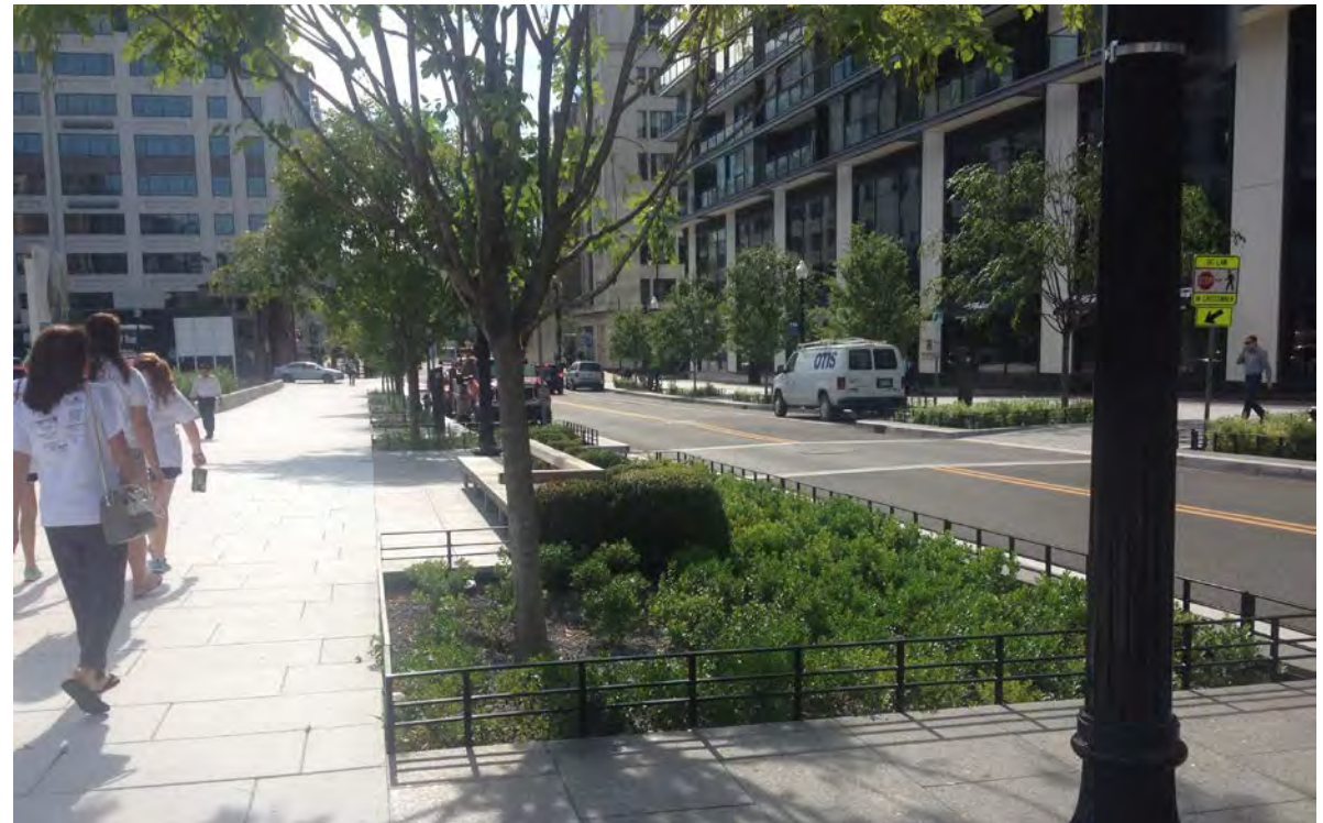
▲ Generous size planting strips and structural soil may be needed to allow large canopy street trees in urban conditions to thrive.
