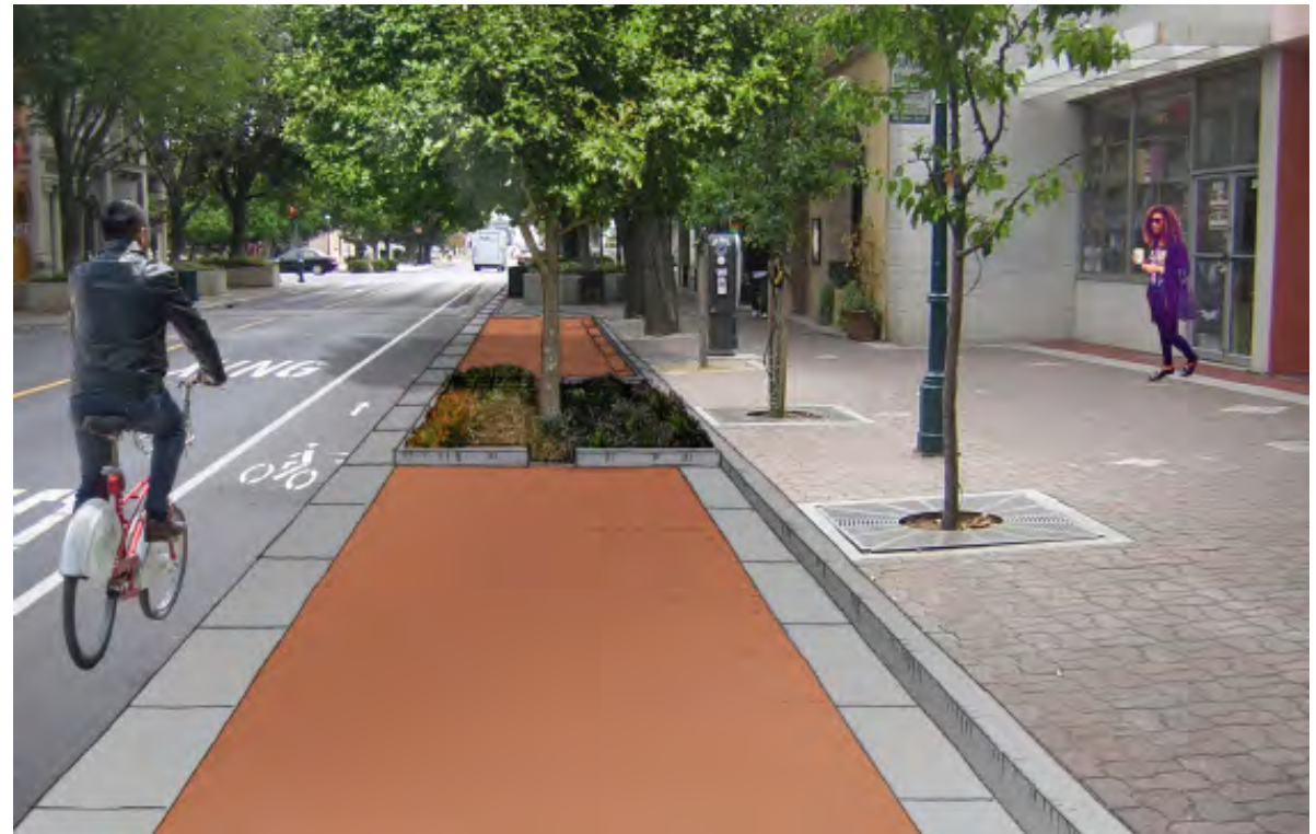
▲ RETROFIT OPPORTUNITY: The same commercial street with a combination of stormwater curb extensions and pervious paving in the parking lane.
