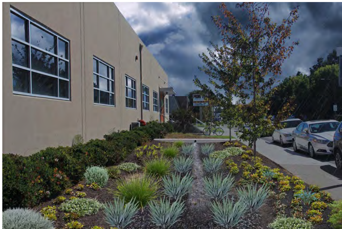
▲ RETROFIT OPPORTUNITY: The same office perimeter landscape converts un-watered grass areas into a rain garden with drought-tolerant landscaping. Roof downspouts direct water into the rain garden.
