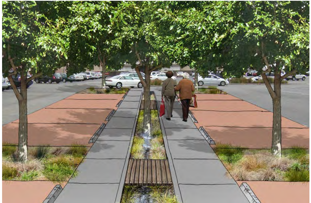
▲ RETROFIT OPPORTUNITY: The same parking lot retrofitted with a stormwater planter/vegetated swale. Notice the sidewalk zones and dedicated crossings to allow for adequate pedestrian circulation.
