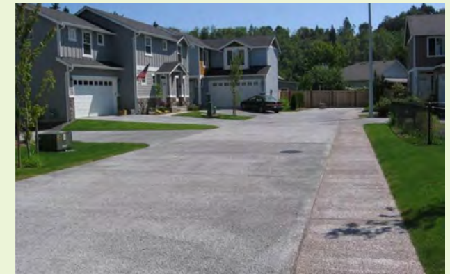
▲ Pervious pavements such as pervious concrete can be used in different land uses and street types. Different colored pavements can be used to define pedestrian and vehicular spaces.
