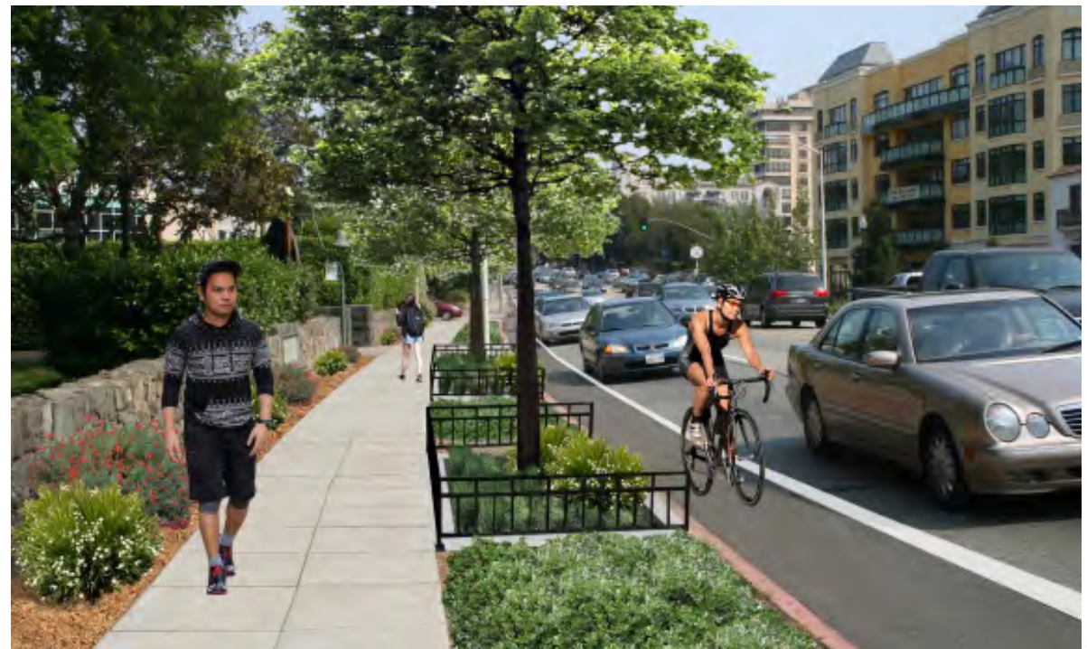
▲ RETROFIT OPPORTUNITY: The same commercial street with tree well filters to capture and treat stormwater runoff and bike lanes to define space for cyclists.
