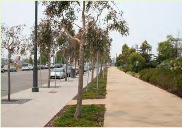
▲ This green gutter captures stormwater runoff from a regional bike path and provides a vegetated buffer between a sidewalk.
