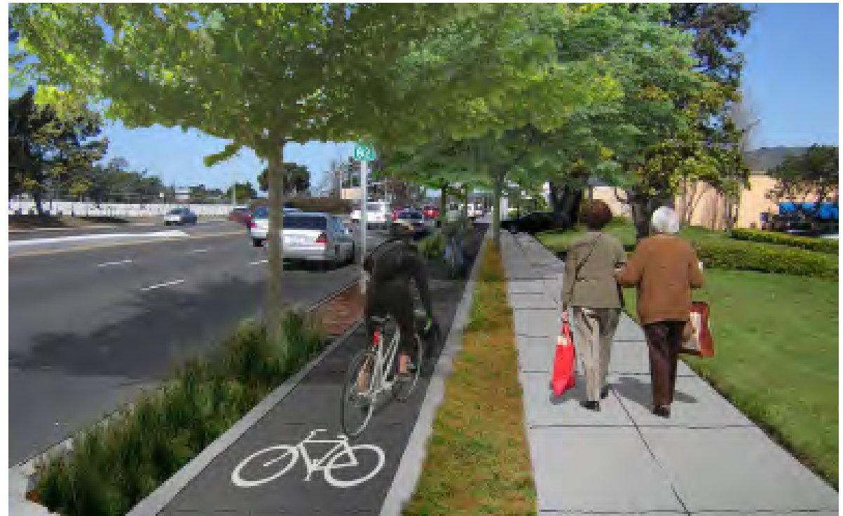
▲ RETROFIT OPPORTUNITY: The same street retrofitted with a series of stormwater planters and pervious pavement, a separated cycle track, and additional street trees.
