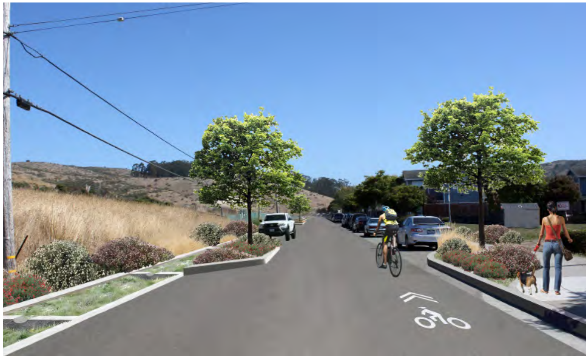
▲ RETROFIT OPPORTUNITY: The same street with a combination of terraced stormwater planters and stormwater curb extensions.
