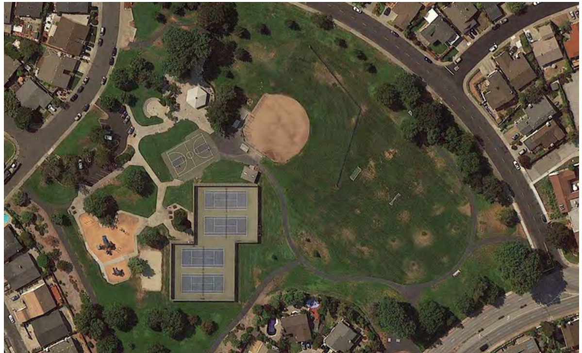
▲ This aerial photo illustrate the impervious area that generates runoff from a low-density park condition as well as the amount of landscape available to capture stormwater runoff.
