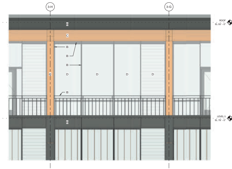
2 Typical Office Enclosure at Terrace - Elevation 3/8" = 1'-0"
