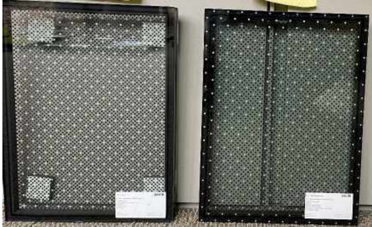
Figure 24. Two preliminary glass samples that combine the dark gray thermal frit and lighter-toned bird-safe frit were reviewed by H. T. Harvey & Associates. The frit on these samples had very good visibility in different lighting conditions due to the contrast between the light and dark frit, and in our professional opinion are likely to reduce bird collisions with the atrium.
