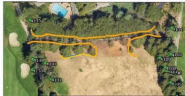
Tree protection fence (gold and enlarged blue) on both sides of the driving range
