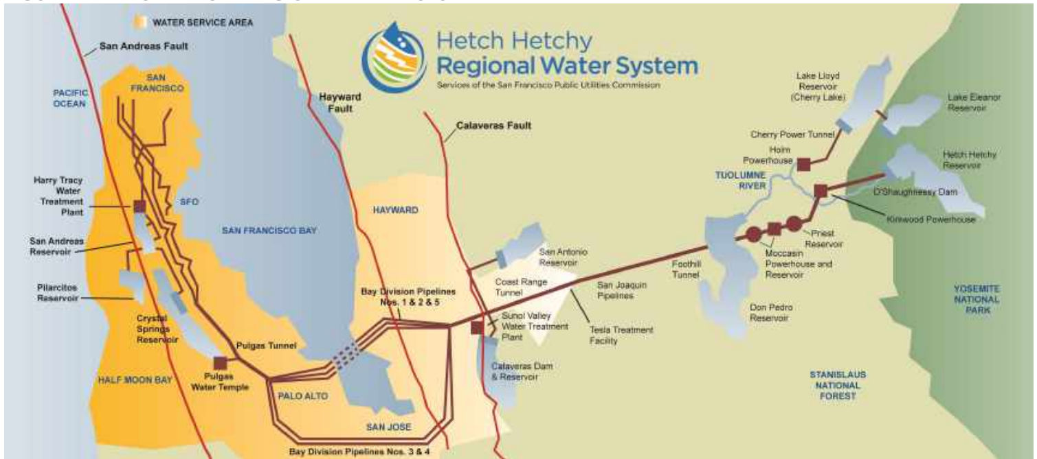
FIGURE 2 - HETCH HETCHY REGIONAL WATER SYSTEM
